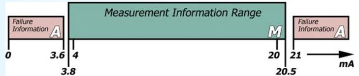
The application should always be configured to detect the current value out of range (<3.6 mA -> 21 mA) and considered "faulty".
